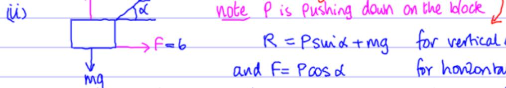
$$R = Psin\alpha + mg \text{ for vertical components}$$
